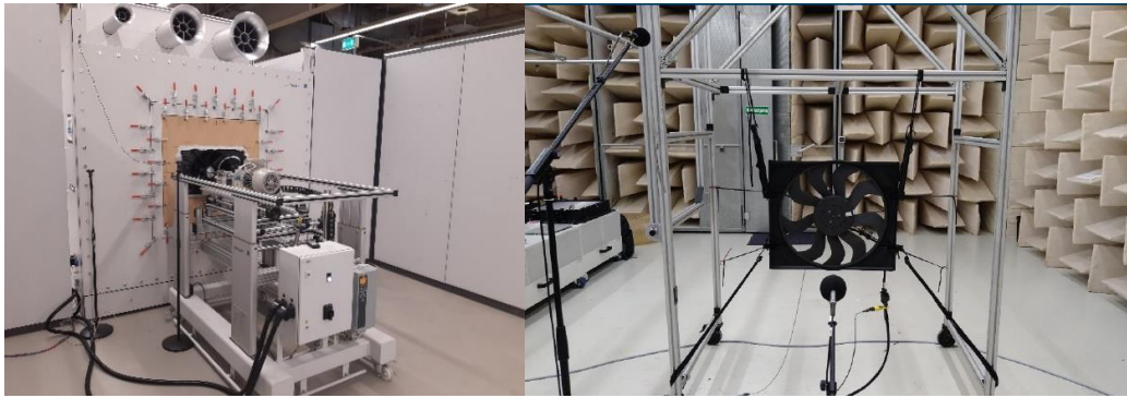
Figure 7: a) ISO 5801 Airflow test stand with external drive at Hanon Systems in Bad Homburg (serial sample is shown) b) Semi-anechoic room with sample fan and two microphones (Hanon Systems, Kerpen, Germany)
