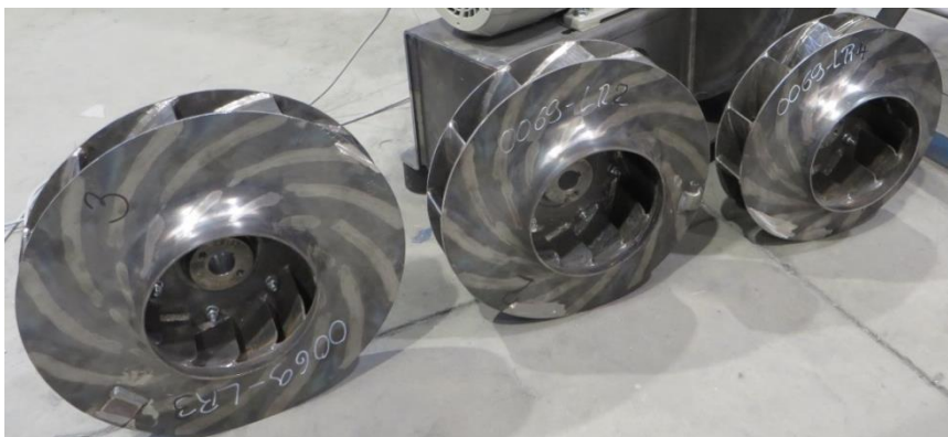
Figure 3: three impellers with different blade length and outlet diameter (from left side: LR3, LR2 and LR4 impellers)
