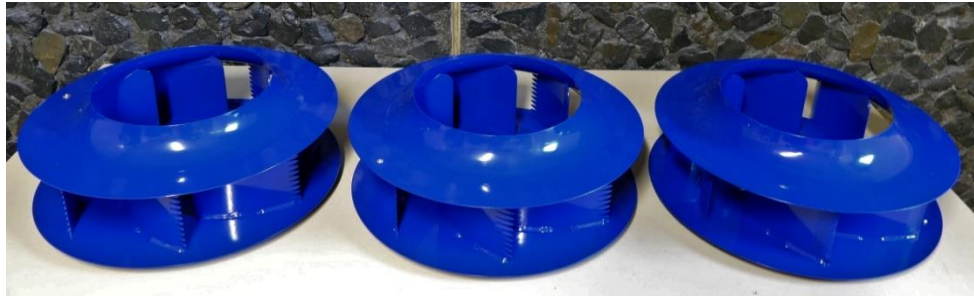
Figure 3: Prototypes of impellers with trailing-edge serrations
