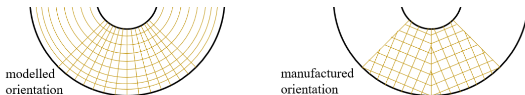
Figure 6: different orientation of fibres in simulation (left) and experiment (right)
