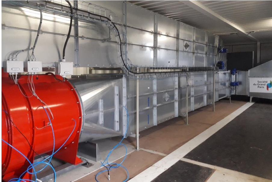
Figure 4: the piston effect test bench – Eiffage, France
