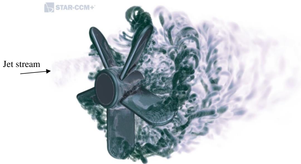
Figure 1: Fan geometry under impinging jet and \lambda_2 vortex criterion plots
