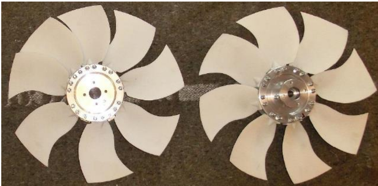
Figure 2 : On the left photo of the disordered blade (“VDP1”), on the right the regular fan (uniformly distributed blades, “Reg”)
