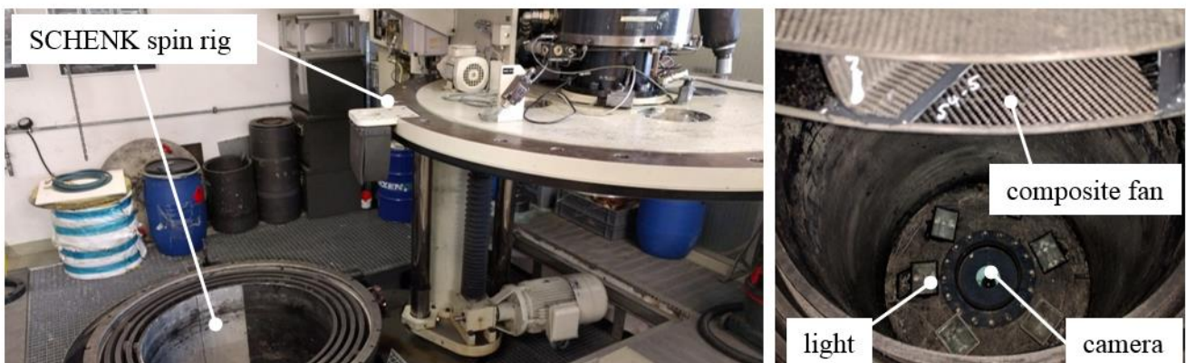
Figure 8: test set-up – SCHENK spin rig (left) and mounted composite fan (right)
