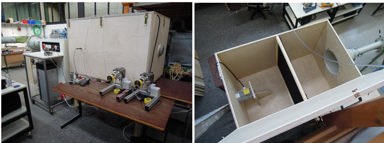
Figure 3: Test airway for volume flow measurement, [6]
