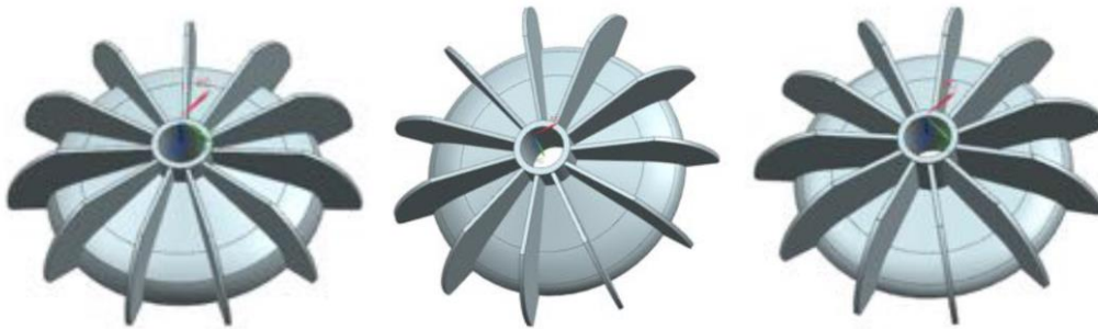
Figure 12: LR-11 impellers with different blade height
