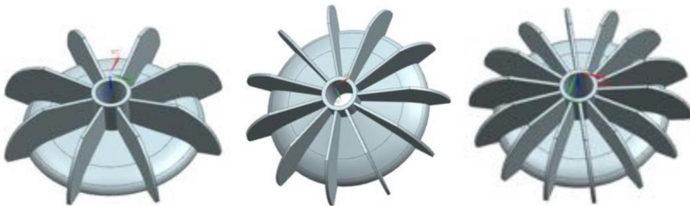
Figure 8: LR-type impellers with different blade numbers
