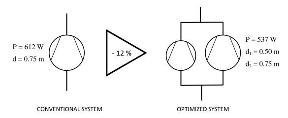
Figure 3: Optimized energy efficient design.
