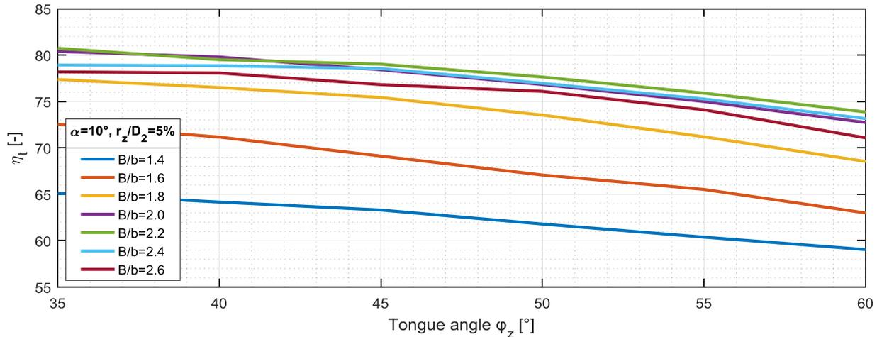
Figure 6: Total efficiency of volutes for different width scale  $B/b_2$  function of tongue angle  $\varphi_z$
