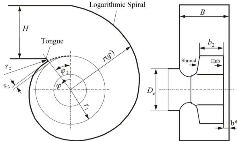
Figure 1: Geometry parameters of spiral casing (Carolus 2013) [3]
