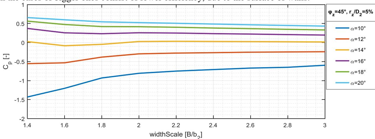
Figure 4: Static pressure recovery coefficient of volutes for different alpha angle function of width scale  $B/b_2$
