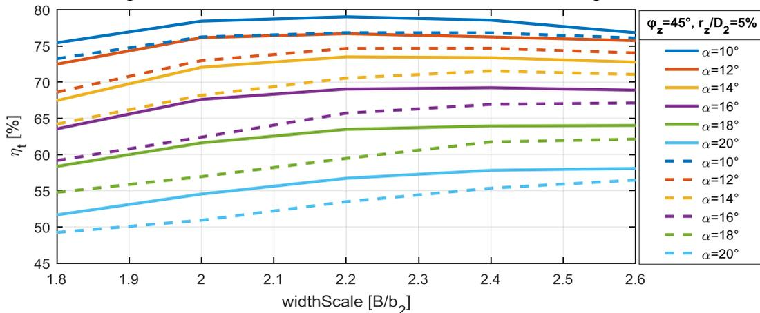
Figure 12: Comparison efficiency of volute with uniform (solid lines) and non uniform inlet velocity (dashed lines).
