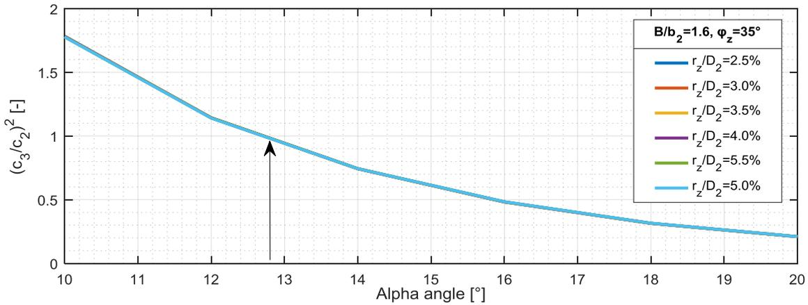
Figure 10: Outlet/inlet ratio of kinetic energy of volutes for different tongue radius  $r_z / D_2$  function of alpha angle. From graph 10 for alpha over  $12.8^\circ$  the ratio of kinetic energy is below value 1.
