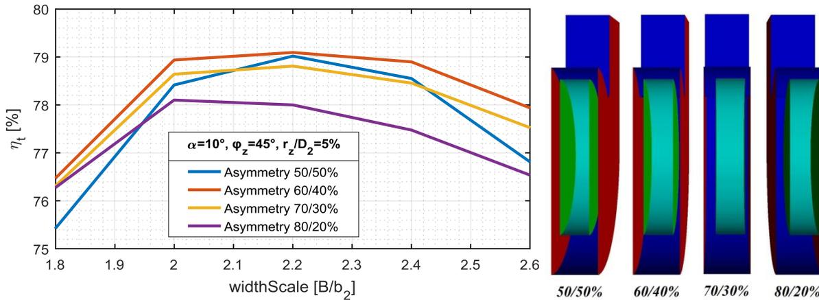
Figure 14: a) Total efficiency of volutes for different position of impeller b) Schematic view of impeller/volute position
