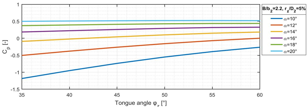
Figure 7: Static pressure recovery coefficient of volutes for different alpha angle function of tongue angle  $\varphi_z$
