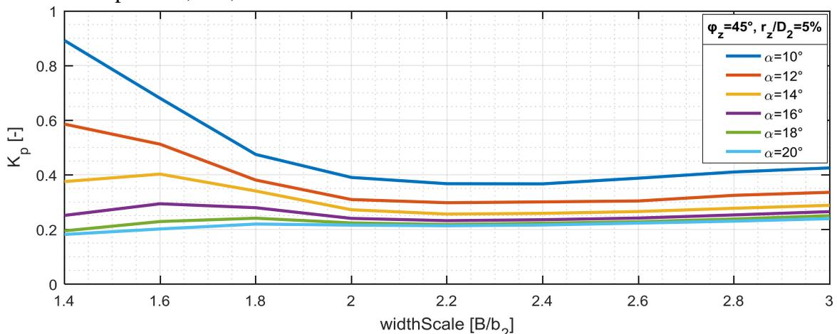
Figure 5: Total pressure loss coefficient of volutes for different alpha angle function of width scale  $B/b_2$
