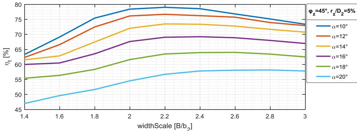
Figure 3: Comparison total efficiency of volutes for different alpha angle function of width scale  $B/b_2$
