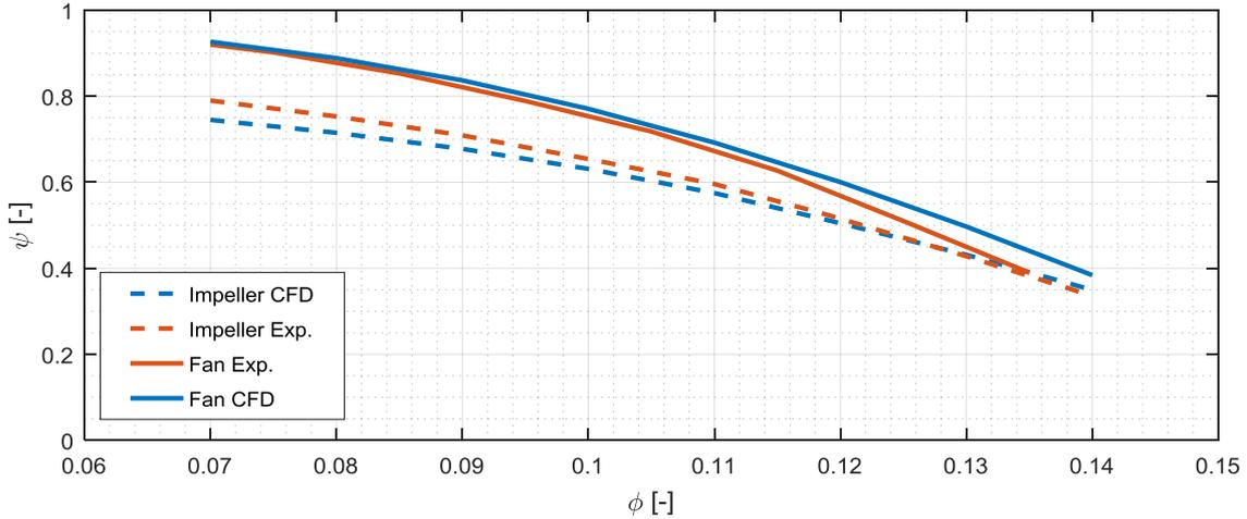
Figure 15: Comparison results from experiments and CFD for impeller and for the complete fan.
