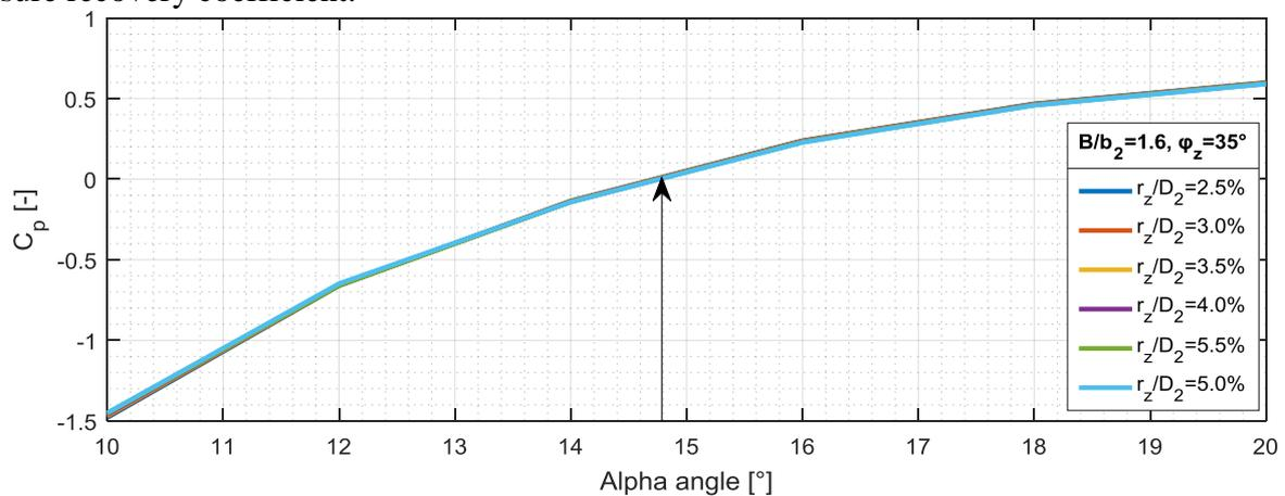
Figure 9: Static pressure recovery coefficient of volutes for different tongue radius  $r_z / D_2$  function of alpha angle .
