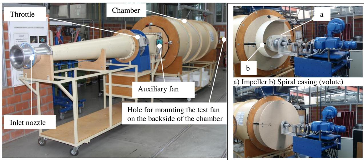
Figure 2: Chamber test rig for the measurement of characteristic fan curves at the University of Siegen. [15]
