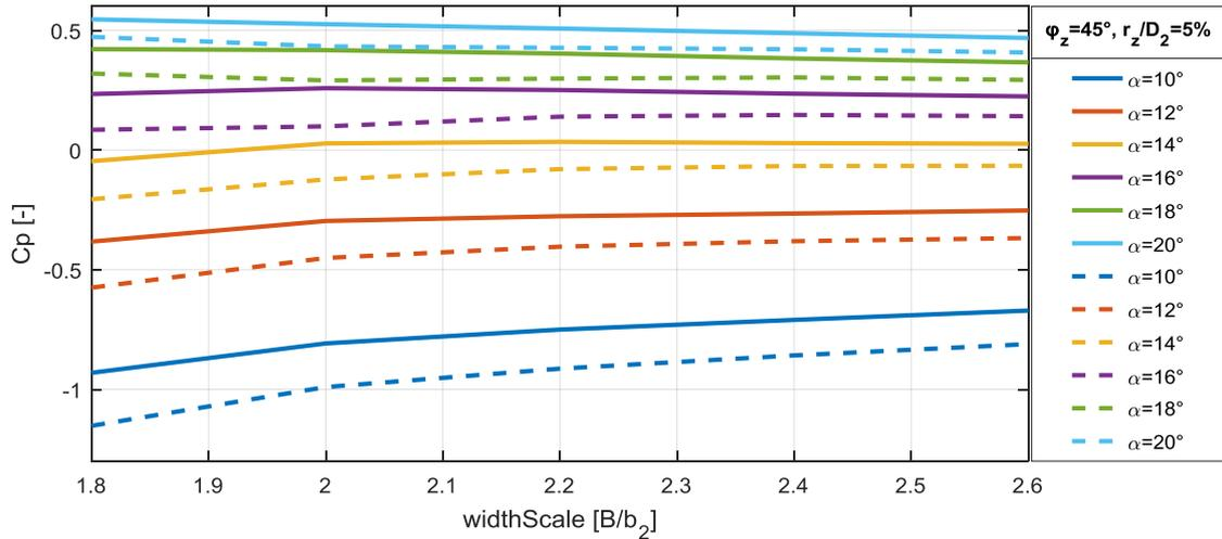
Figure 13: Comparison static pressure recovery coefficient of volutes with uniform (solid lines) and non uniform inlet velocity (dashed lines).
