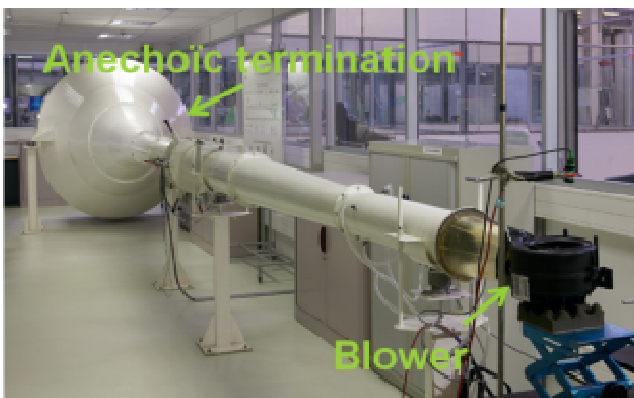
Figure 8: test rig facility at LVR
