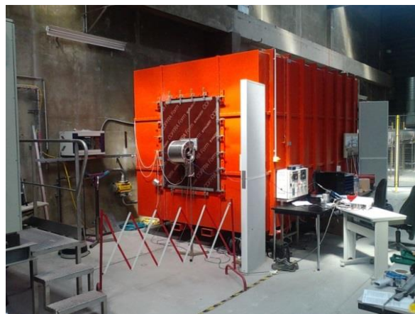
Figure 2: Fan fitted to the pressure chamber
