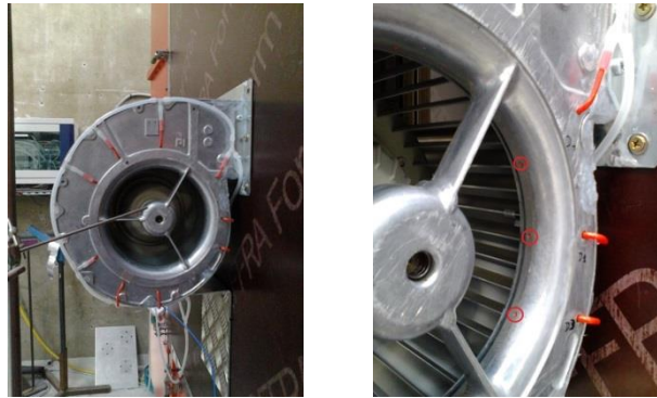
Figure 3: Layout of the pressure taps on the right inlet nozzle
