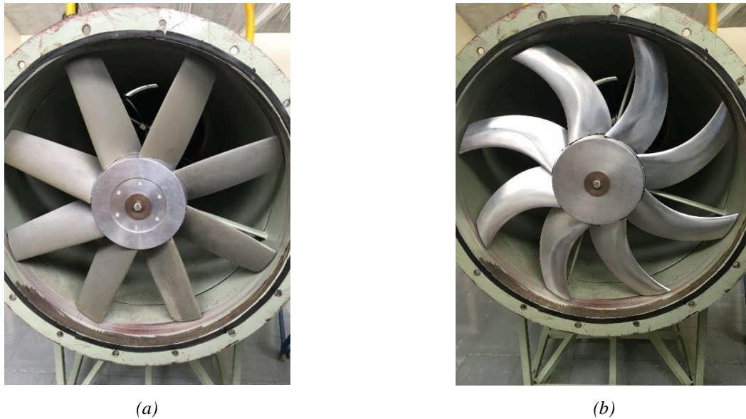
Figure 1 – 630 mm diameter test fans with straight blades, R-fan, (a) and forward swept blades, FS-fan (b).
