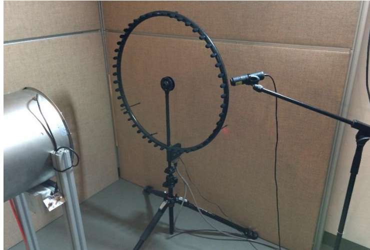
Figure 6: microphone array in front of the pressure side of the CRF
