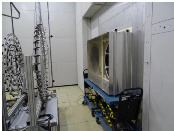
Figure 1: investigated fan configuration: fan in box with microphone array
