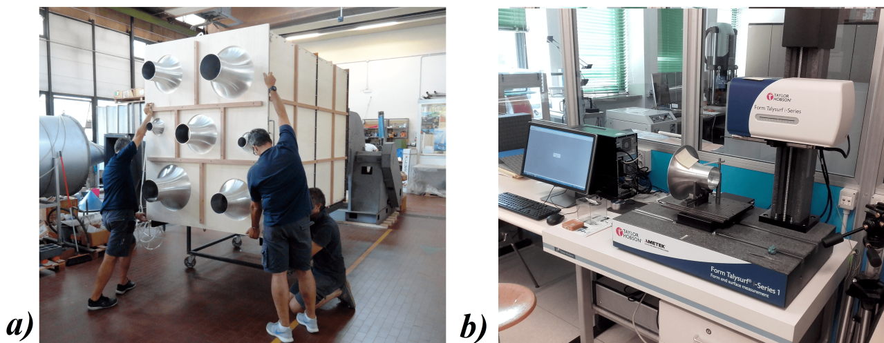
Figure 4: a) The installation of the multi-nozzle wall featuring the symmetrical allocation. b) Metrological tests to determine whether the nozzle’s surface is in compliance with the tolerances.
