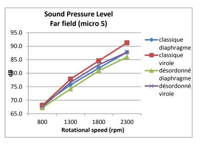
Figure 4: Graph of the sound pressure levels as a function of speed
