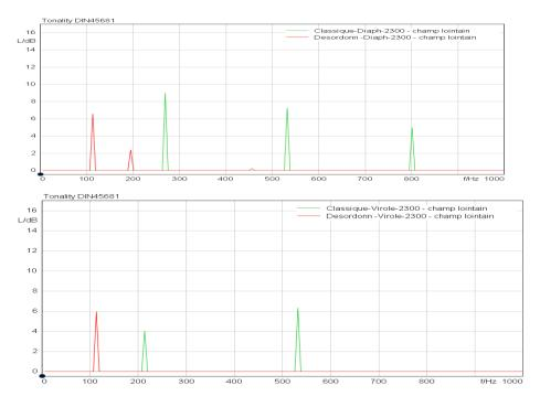
Figure 7 : Tonality - comparison of conventional propeller and propeller with irregularly spaced blades - Diaphragm (top) and Shell (bottom) 2300 rpm
