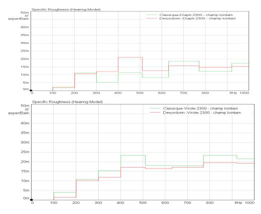
Figure 8 : Roughness - comparison of conventional propeller and propeller with irregularly spaced blades - Diaphragm (top) and Shell (bottom) 2300 rpm
