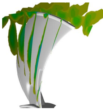
Figure 10: CFD simulation of losses at the blade tip & the positive effect of Winglets on the overall noise level
