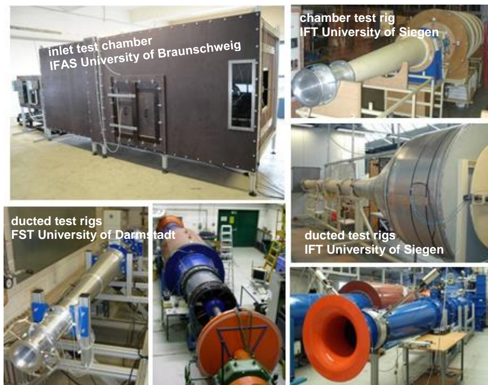
Figure 6: Air Performance Test Rigs according to ISO 5801 [1] and ISO 13347 [2]
