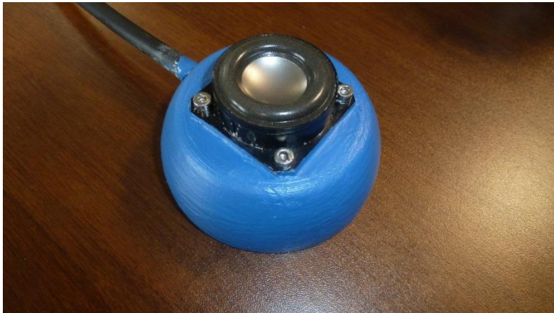
Figure 8: Photograph of the designed loudspeaker
