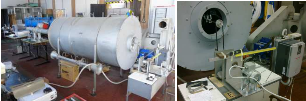
Figure 2: The ISO 5801 category A fan test rig (on the left) and the torsion balance (on the right) used for the experimental tests
