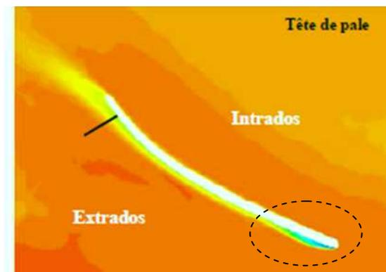
Figure 4- RANS calculation of the flow around a blade, showing the recirculation bubble
