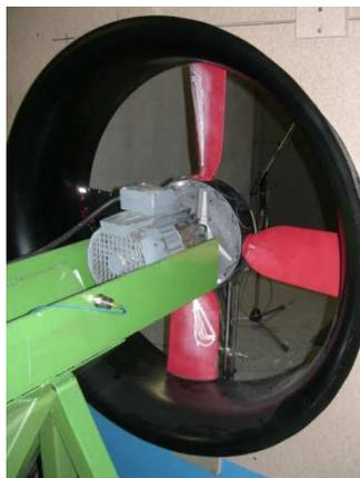
Figure 1 – Experimental fan in 4 blades configuration with a shroud (doc. CETIAT)
