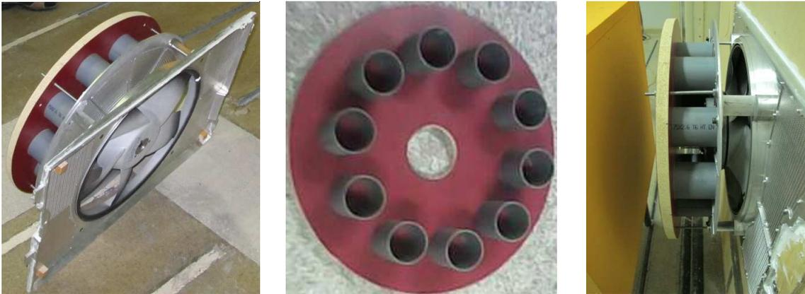
Figure 12. Semi – radial fan with, MPP shroud and MPP back plate fitted with QWRs. QWR dimensions; inner diameter 100 mm, height 80 mm, covered with MPP with, thickness 1 mm, slit width 0.2 mm and 1% porosity. QWR covered area is 40% of the total back plate area.
