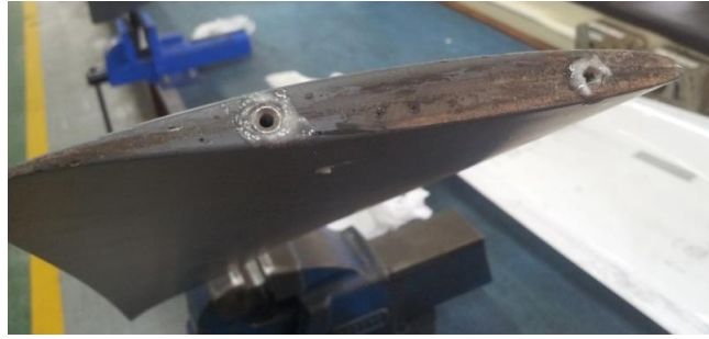
Figure 2: Blade tip mounting points at the blade tip
