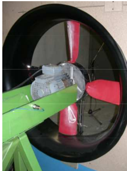
Figure 2 Experimental set-up. The unsteady pressure sensor are visible on the upper and lower blade.
