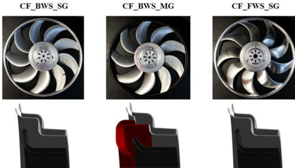
Figure 3: Investigated axial cooling fans with different gap geometries
