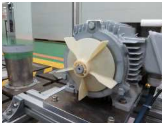
Figure 1: Bi-directional radial fan of the industrial motor (without fan cover)
