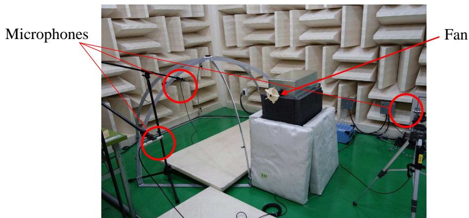
Figure 7: Measurement environment in the semi-anechoic room
