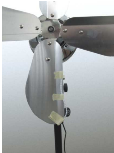
Figure 2: Fan with applied disturbance (ball type cable tie) at the trailing edge of the blade at 6 o'clock.
