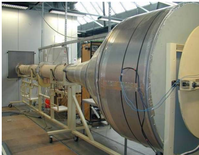
Duct test rig at IFT, diameter 0.3 m
