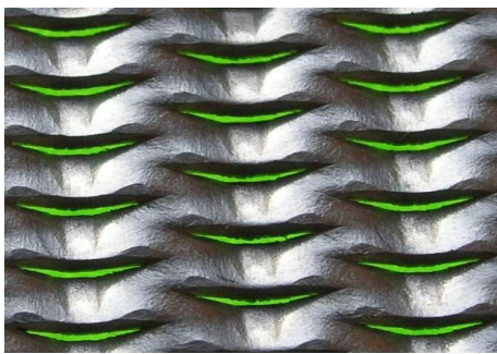
(a) Photo of the MPP used with slits (Acustimet TM ). (b) MPP baffle with rigid inner walls and spacing 165× 241 mm.
