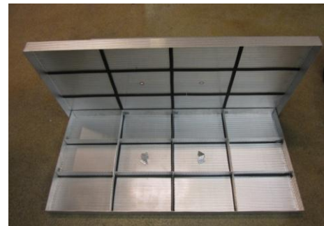
(a) Photo of the MPP used with slits (Acustimet TM ). (b) MPP baffle with rigid inner walls and spacing 165× 241 mm.
