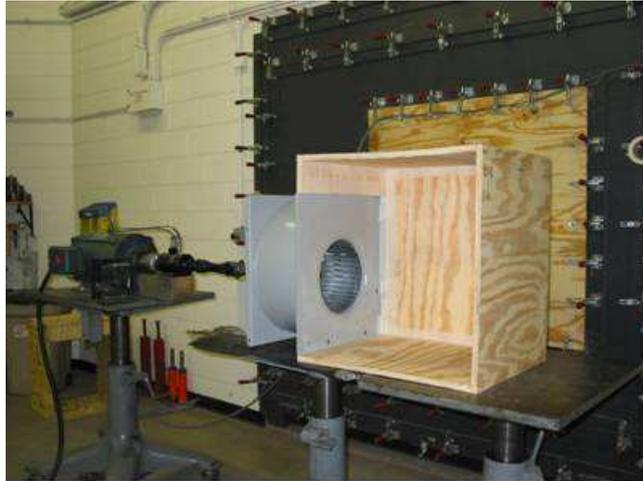
Figure 17: FC centrifugal fan with inlet cabinet 1 (from [7])
