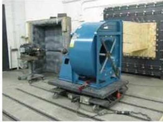
Figure 10: BI centrifugal fan with inlet bearing obstruction (from [6])
