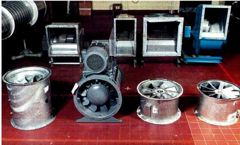
Figure 7: Views of the test fans (from [4])
