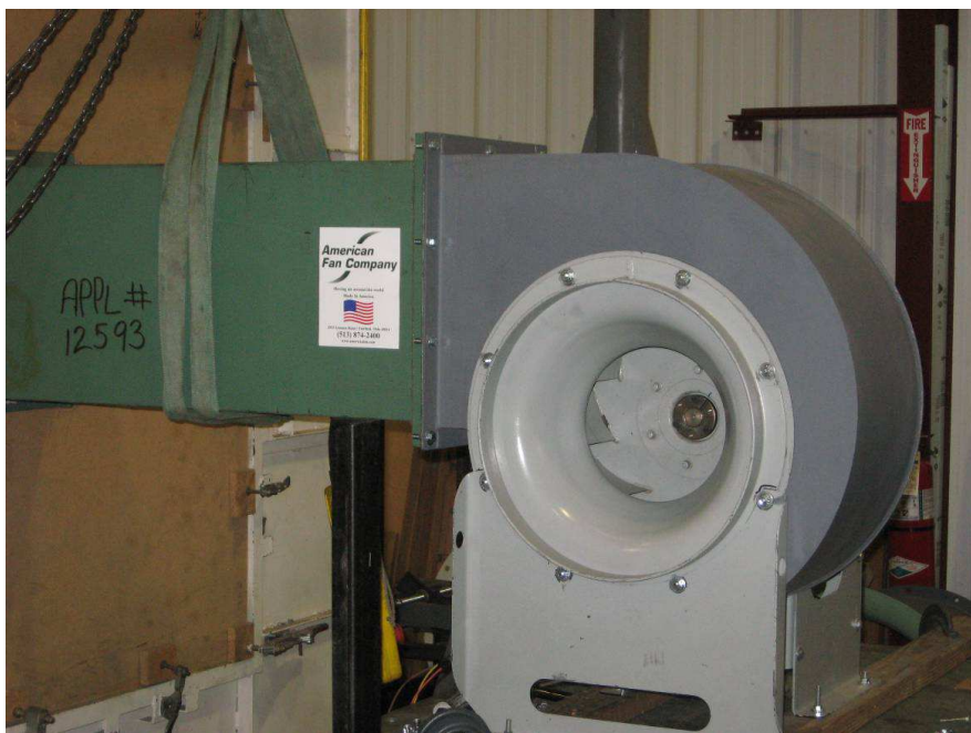
Figure 3 – Test setup to compare performance impact of intermediate shroud; setup per AMCA 210-07, Figure 12, Installation Type B.
