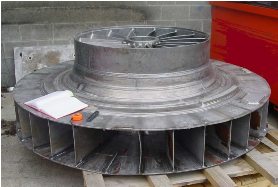
Figure 1 Photograph of the MVR impeller with missing blade
