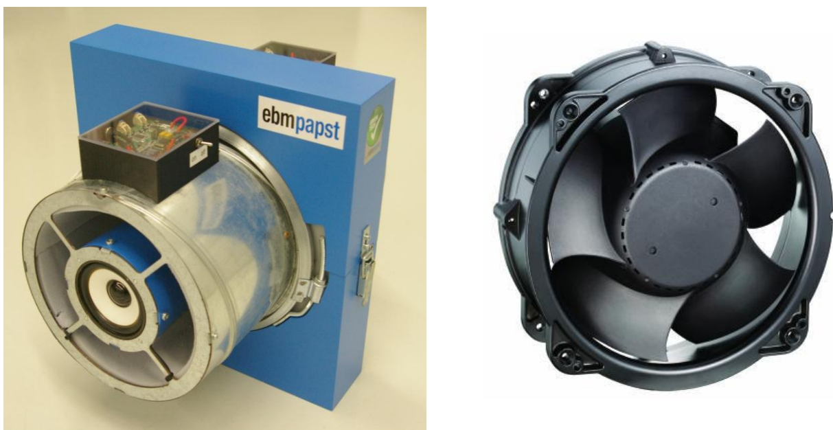
Figure 5: ANC demonstrator (left) with diagonal fan DV6224 (right) inside
