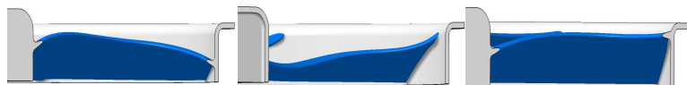
Figure 2 – Left to right: Leading edge of Fan A, Fan B and Fan C.
