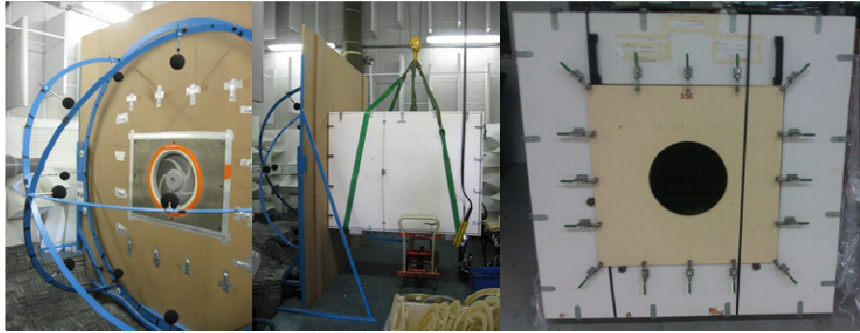
Figure 9 - Left: Reverberant panel with fan and microphones. Center: Flow-rate control rig. Right: diaphragm for flow-rate control.
