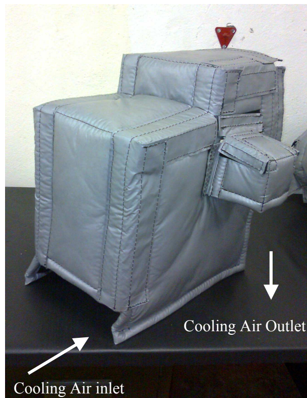
Figure 8: Fan motor jacket
