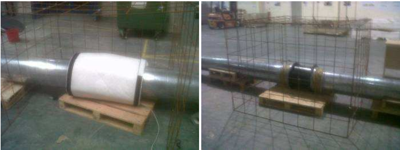
Figure 3: Tested axial fan without and with acoustic jacket; grid indicates locations of the intensity probe
