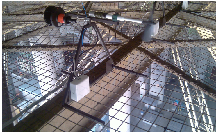
Figure 6: Frame with anemometers and thermocouple
