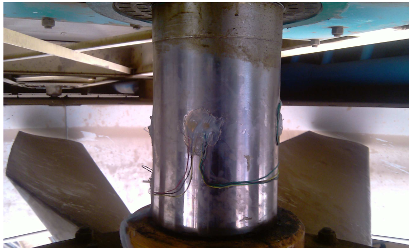
Figure 4: Strain gauge placement on shaft
