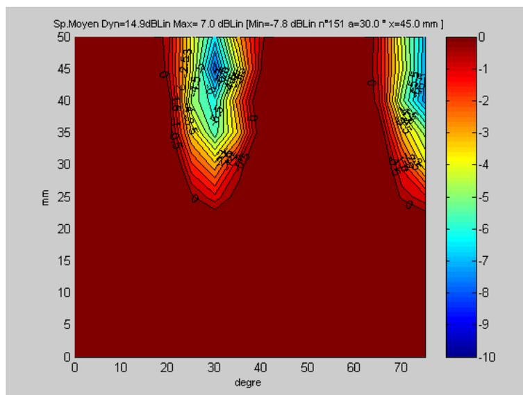
Figure 5- Example of Sound Map (D type with 8 indentations).
