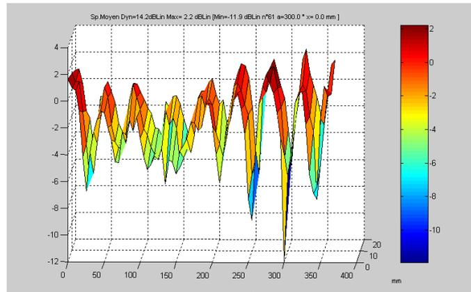
Figure 10- Sound pressure level at BPF for C3 obstruction. Influence of angular and axial position. Horizontal axis is the angle in degrees and the second axis is the distance in mm
