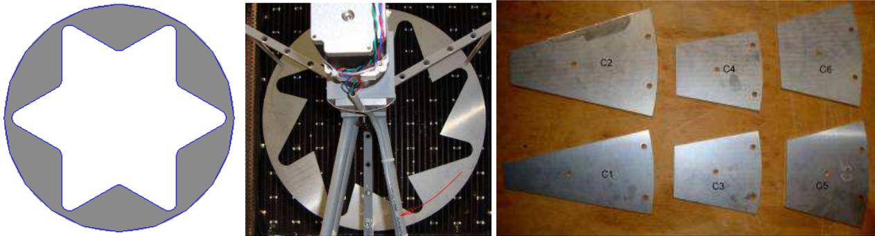
Figure 4- Example of M type (left), D type (center), and C type (right) obstructions.
