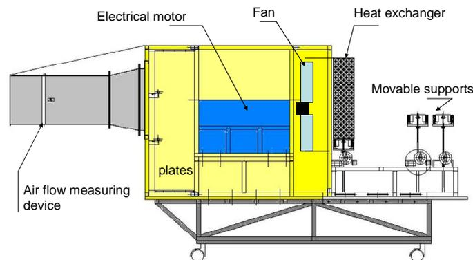
Figure 1- Fan test rig
