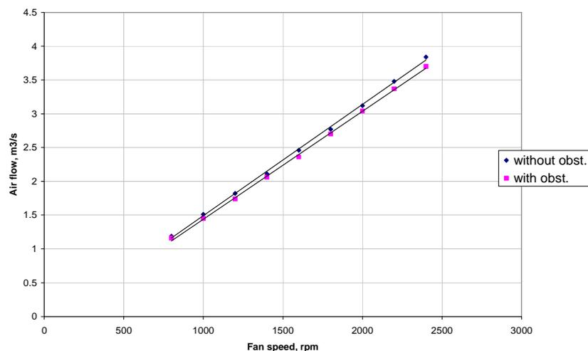
Figure 9- Influence of the obstruction on the flow (M 8 type).
