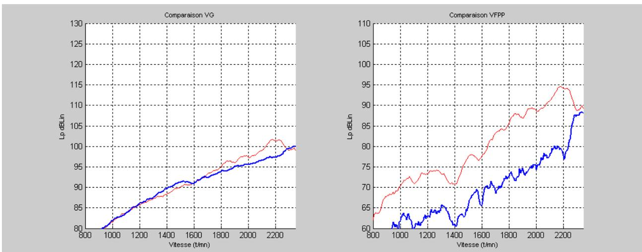
Figure 13- Influence of the fan speed on the overall sound level (left) and at BPF (right). M type obstruction with 6 indentations. Red: without obstruction, blue: with obstruction.
