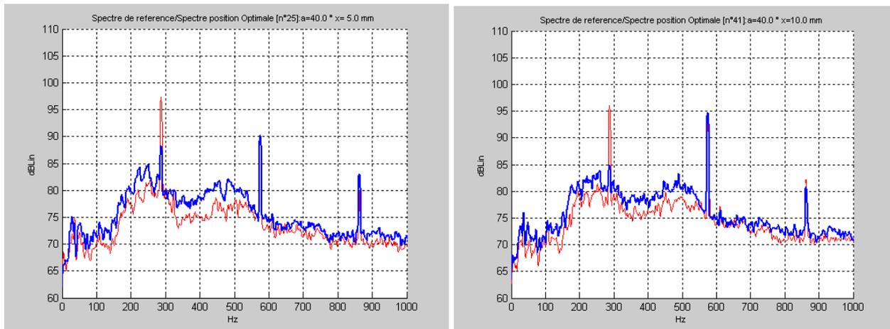
Figure 7- Sound pressure spectrum at optimal location for the best M type (left) and D type (right) obstructions.
