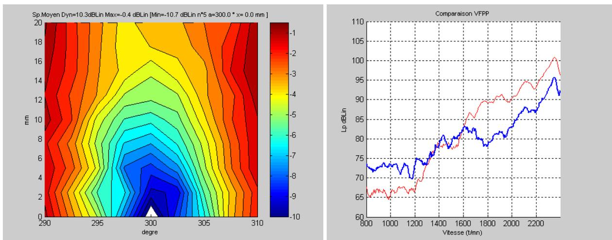
Figure 11- Best C type obstruction (C5). Sound map around nominal position at 2200 rpm (left) and sound level when varying fan speed (right), obstruction at fixed position Red: without obstruction, blue: with obstruction..
