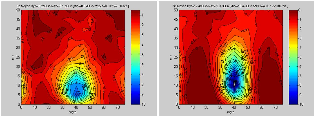
Figure 6- Sound Map obtained with the best M type (left) and D type (right) obstructions.
