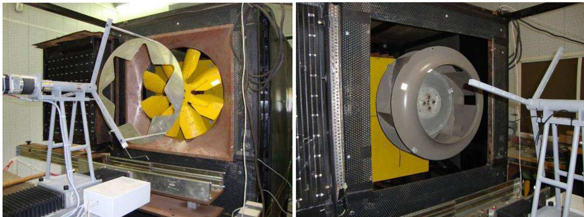
Figure 3- Axial (left) and centrifugal (right) fans.
