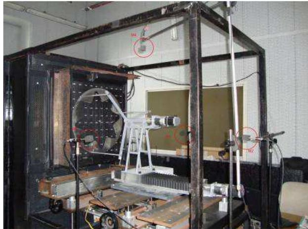
Figure 2- Microphones M1 to M4 location, and automaton.
