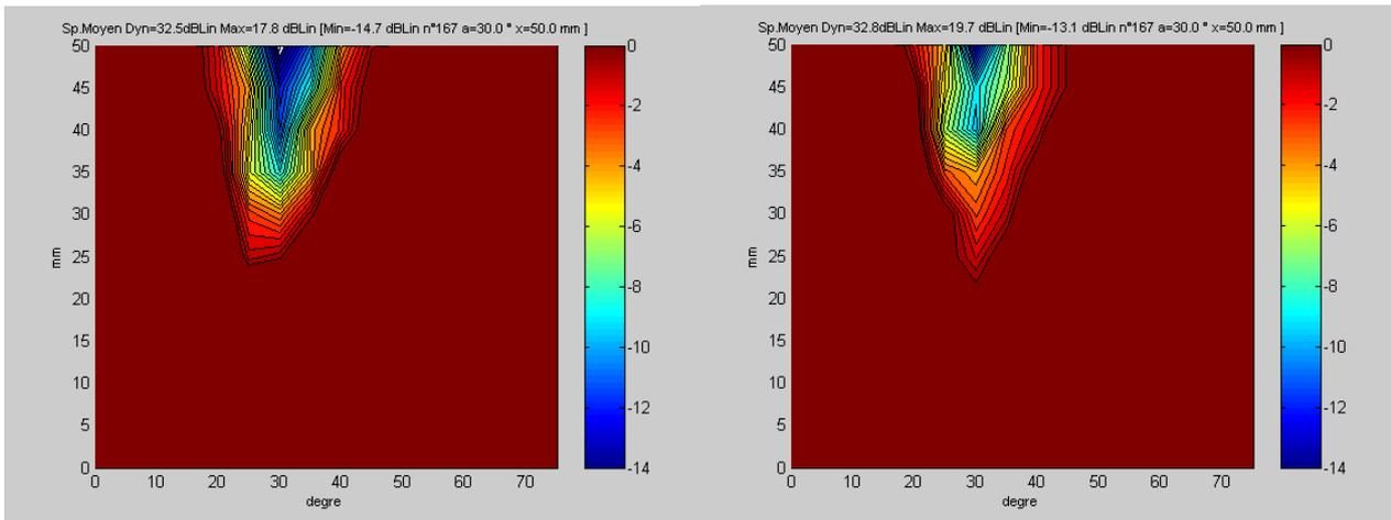
Figure 12- Sound map for the best M (left) and D(right) type obstruction with the centrifugal fan at 2200 rpm.
