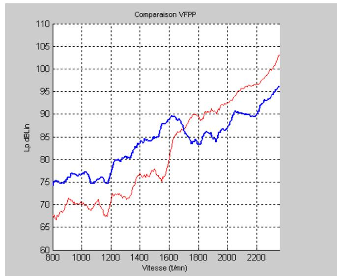
Figure 8- Sound pressure level for an obstruction in fixed position, when varying the fan speed (D 8 type)
